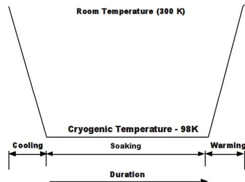
**Figure 4:** Cryogenic Treatment Cycle
