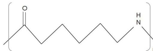
**Figure 2:** Chemical Structure of Nylon 6
