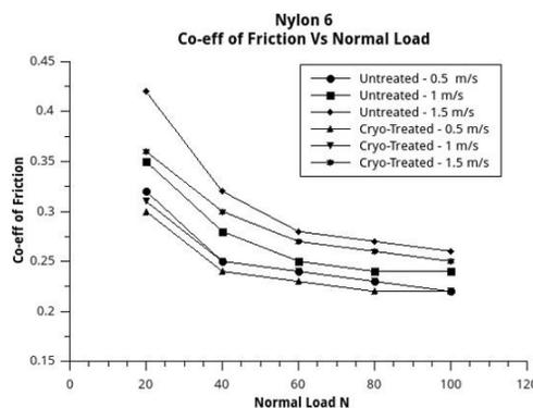
Figure 5: untreated and cryo-treated Nylon 6
