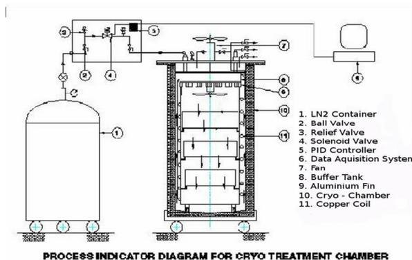
**Figure 3:** Cryogenic Processor
