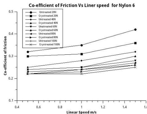
**Figure 7:** untreated and cryo-treated Nylon 6
