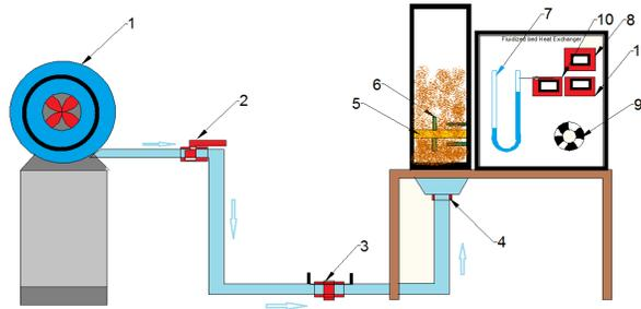
**Figure1 :** 1.Blower,2.Air regulator, 3.Orifice, 4.Funnel, 5.Heater, 6.Thermocouples, 7.Manometer, 8. Temp. indicator, 9.Dimmerstat, 10&11. Voltmeter and Ammeter
