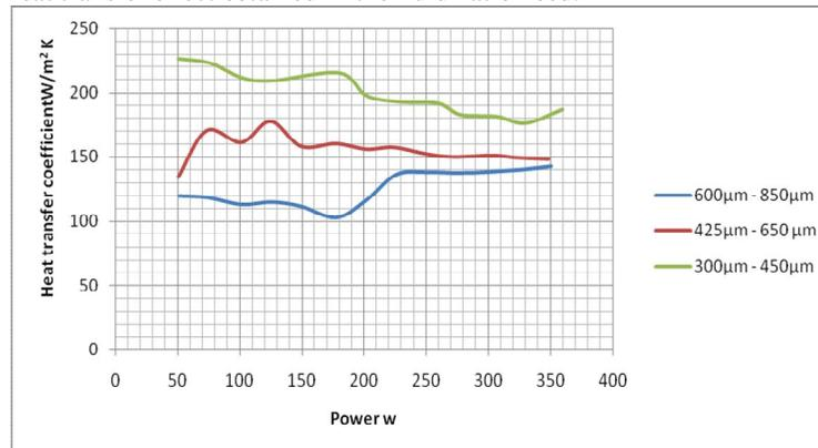
Graph 4: Comparison between heat transfer coefficient and power @velocity of air 4.96 m/s
