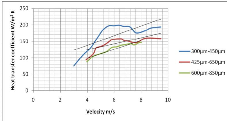
**Graph1:** Comparison between heat transfer coefficient and velocity of air @ 200 watt
