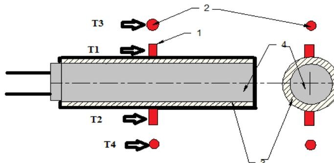
**Figure3:** Shows Thermocouple and Cartridge heater setup inside the chamber.
