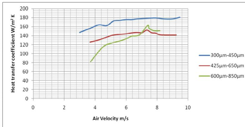
**Graph 3:** Comparison between heat transfer coefficient and velocity of air @ 400 watt
