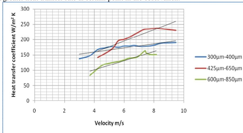
**Graph 2:** Comparison between heat transfer coefficient and velocity of air @ 300 watt
