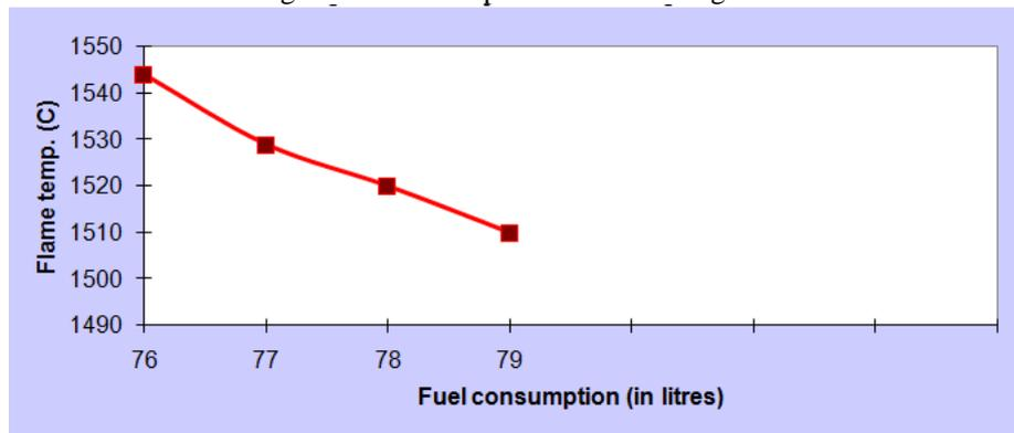
Fig.4 -- Flame Temperature Vs fuel consumption
